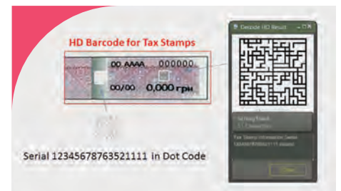
Fig 2 – HD Barcode for tax stamps with dot pattern
